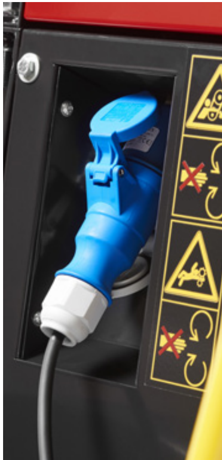
Integrated charger: 230V 16A 65V and cable
