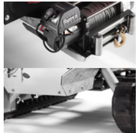
TP winch for climbing steep grounds. Best Ground clearance on market: 200 mm Track width: 1150-1300 mm. Reinforced hose protection.
